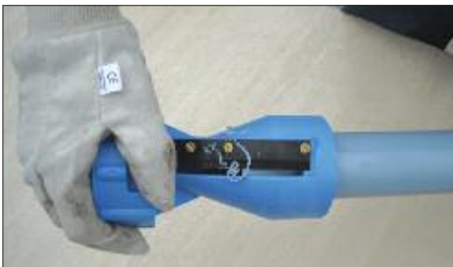
3. Chamfer end of pipe using a chamfering tool or file. 用倒角器或銼刀將管件倒角
